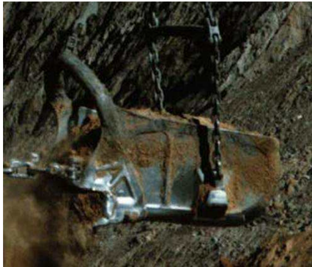
A normal dragline bucket shows a flat payload profile when operating in common low cohesive materials:
