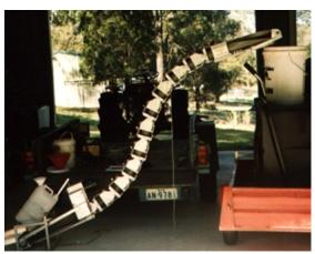
The photos show a bench test of fine phosphate sand material being conveyed at 70 degrees through two tight vertical curves. CAP equipment has the capacity to replace some bucket elevator applications.
