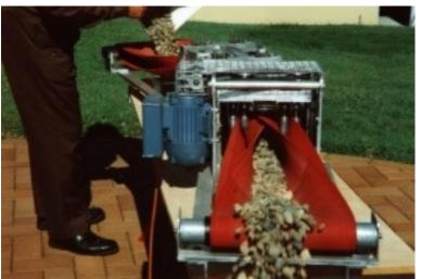
The CAP was initially designed for mining use where the idler bearing frame can be bolted to the side or the drive roof. Alternatively it may be supported by a trolley running on an overhead "I" beam, as is now commonly installed in coal mine development drives. The latter option means the CAP can be retracted and advanced from the tunnel face as soon as an I-beam extension is installed.
