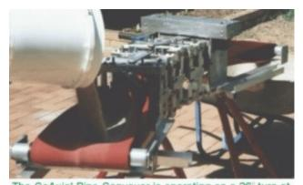
The CoAxial Pipe Conveyor is operating on a 26° turn at a 20:1 pipe diameter to curve radius..
