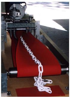
These photographs show some detail of our driven idler arrangement. After much bench testing and confirmation mechanical stress calculating, we have designed the driven idler spring shown above. This drive spring completed over ten million cycles, which surpasses the British standard for an infinite spring life, and we are therefore very confident that the idler drive system is a reliable, cheap, and an effective way to power a coaxial pipe conveyor belt.
