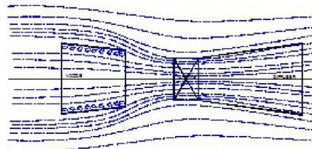
A combined nozzle, turbine and diffuser assembly is called a Fuselage Turbine (FT), as illustrated.
