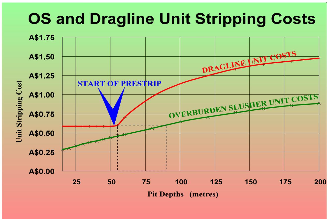
Dragline unit costs at 55m depth (60.3¢/bcm) match the OS at 90m. Put another way, a large dragline stripping 14,430,000bcm<sub>pa</sub> at 55m pit depth, costs \$8,700,000<sub>pa</sub> to operate. An OS system, shifting the same overburden, has operating costs of \$6,700,000<sub>pa</sub>. **The lower OS stripping cost amounts to a saving of \$2,000,000<sub>pa</sub>, or 23%.** However, there are also productivity improvement opportunities.
