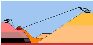
An OVERBURDEN SLUSHER starts strip-mining following the ground preparation. Where this involves drill and blast, the HOE starts stripping directly on top of the shot rock, without the need for pre-levelling. The LW pulls the HOE forward to fill and then transport the load through to the spoil bank, on an underlying shear-plane. Drag ropes then slacken, stopping the HOE. The payload develops passive resistance across the underlying shear-plane. The
