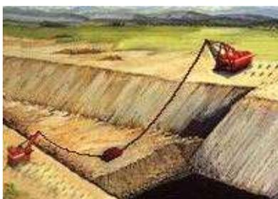
When the block is complete, the OVERBURDEN SLUSHER moves down the pit to the next block, which is about 30m along the strike. Stripping proceeds until the current strip horizon of coal is uncovered. Coal is then extracted, and the OVERBURDEN SLUSHER returns to remove another layer of waste - either as parting down to the next coal seam, or overburden in the next strip.
